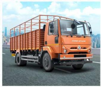
According to the company, the latest version of the i-Gen6 technology 150 HP engine powered vehicle is available in 11T, 12T,14T and 16T GVW haulage segment and 5-6 cum tipper segment with 6-speed overdrive gearbox and optimised gear ratios options to suit all haulage and tipper applications
