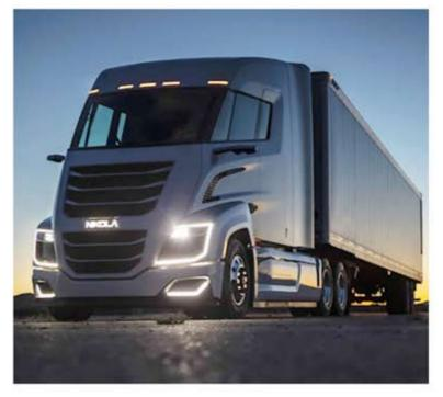
The company's Tre battery-electric vehicle (BEV) variant currently covers up to 300 miles.
