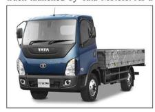
commercial vehicle, it became known for its exceptional quality of materials. This model produces over 98 horsepower of torque, enough to perform many functions. It has a payload capacity of 3692kg and also meets BS VI emission standards.
